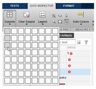
After you create the plots, the BrakeAssertion signal stays in the first plot. Click a plot where you want a signal to appear and then click the signal. Using this technique, add Input 3 (brake input) in plot 2 and throt in plot 3.
