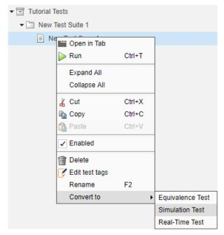
**5** Rename the test My Verification Test. You can use the context menu in the test browser and select **Rename**. Or, you can click the name and type a new one in the test case.
